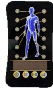
Touch module with Glass + multi color silk screen printing used in medical devices
