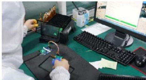
TP Functional testing
